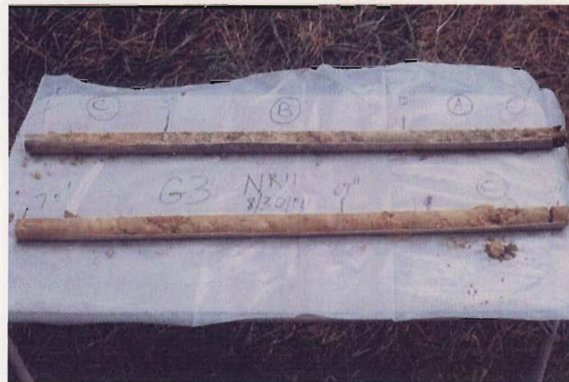
Photo. C-24 Groseclose and Poplimento Silt Loam soil profile: surface (A horizon) and subsurface (B and C horizons) for sample location NRUG3
