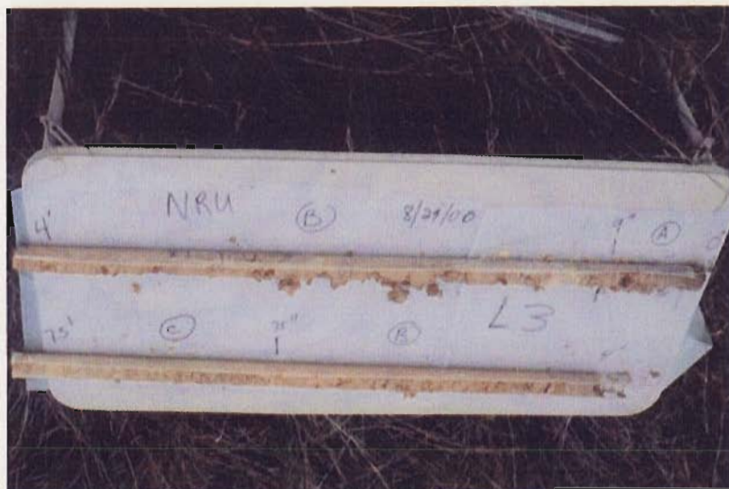
Photo. C-29 Lowell Silt Loam soil profile: surface (A horizon) and subsurface (B and C horizons) for sample location NRUL3
