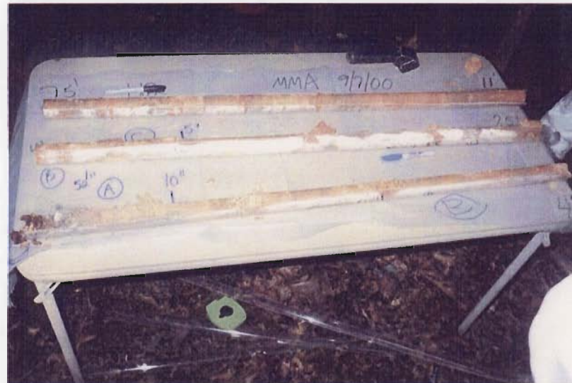
Photo. C-8 Unison-Urban Complex soil profile: surface (A horizon) and subsurface (B and C horizons) for sample location MMAU2
