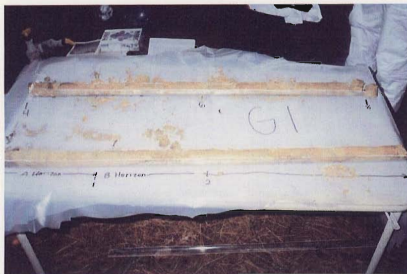
Photo. C-23 Groseclose and Poplimento Silt Loam soil profile: surface (A horizon) and subsurface (B and C horizons) for sample location NRUG1
