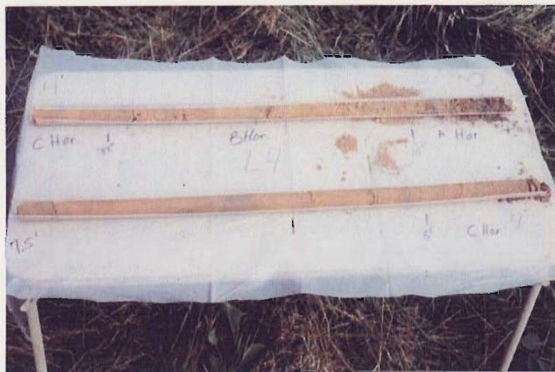
Photo. C-31 Lowell Silt Loam soil profile: surface (A horizon) and subsurface (B and C horizons) for sample location NRUL4
