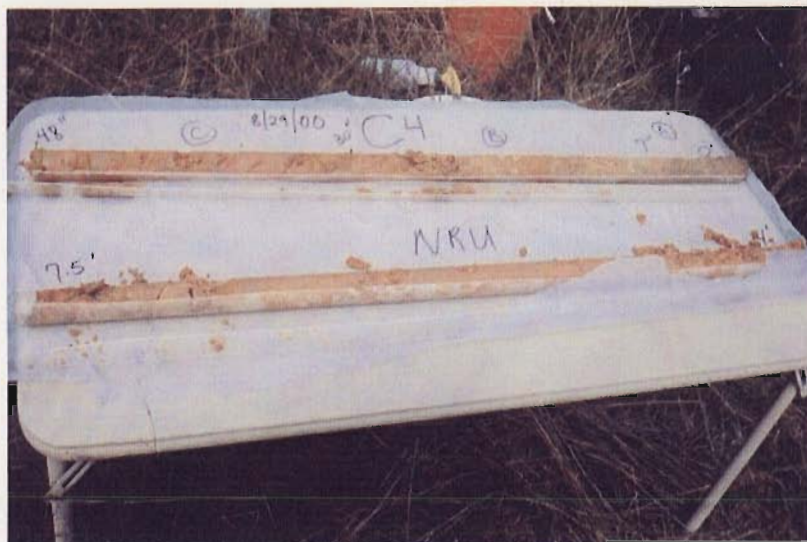
Photo. C-21 Carbo Silty Clay Loam soil profile: surface (A horizon) and subsurface (B and C horizons) for sample location NRUC4
