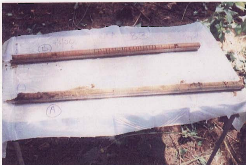
Photo. C-3 Braddock Loam soil profile: surface (A horizon) and subsurface (B horizon) for sample location MMAB3
