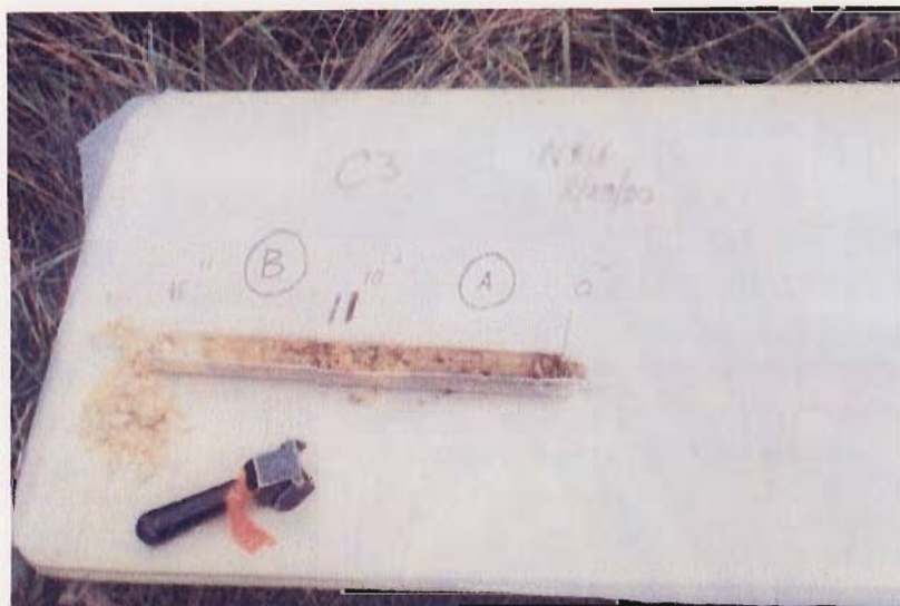
Photo. C-19 Carbo Silty Clay Loam soil profile: surface (A horizon) and subsurface (B horizon) for sample location NRUC3
