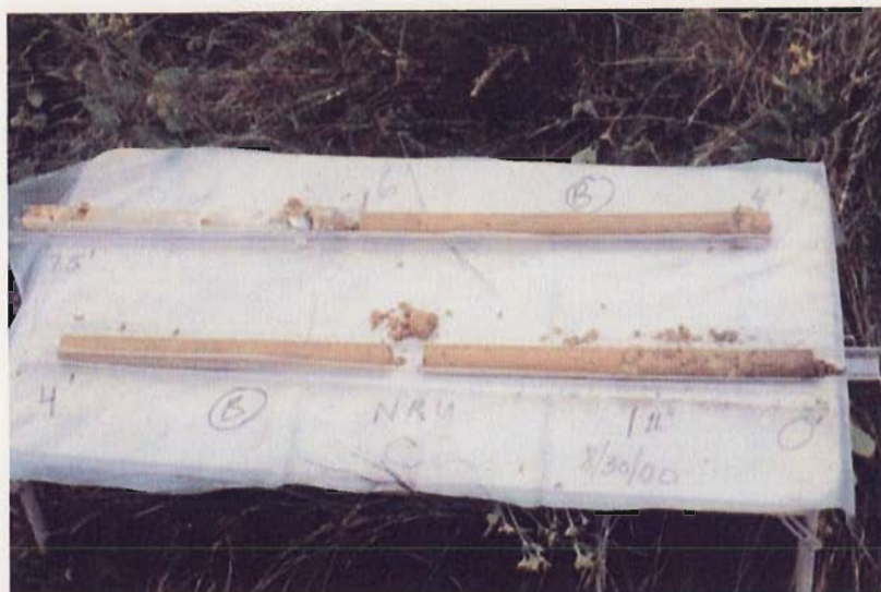
Photo. C-17 Carbo Silty Clay Loam soil profile: surface (A horizon) and subsurface (B horizon) for sample location NRUC2
