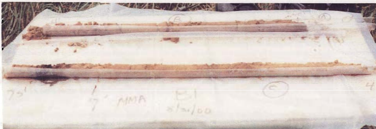
Photo. 2 Braddock Loam soil profile for sample location MMAB1: surface (A horizon) and subsurface (B and C horizons) collected from the MMA
