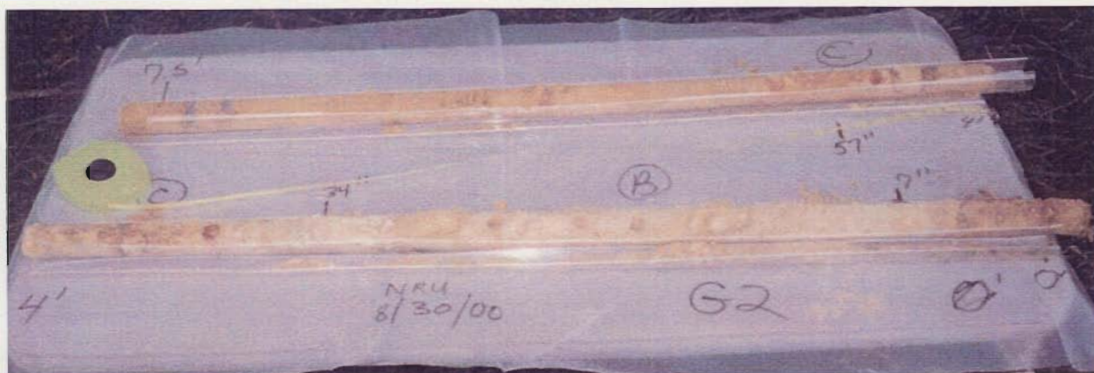
Photo. 10 Groseclose and Poplimento Silt Loam soil profile for sample location NRUG2: surface (A horizon) and subsurface (B and C horizons) collected from the NRU
