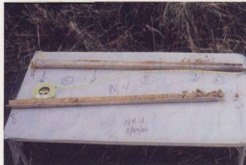
Photo. C-36 Wurno-Newbern-Faywood Silt Loam soil profile: surface (A horizon) and subsurface (B and C horizons) for sample location NRUW4
