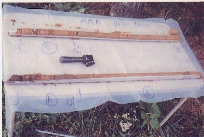
Photo. C-13 Wheeling Sandy Loam soil profile: surface (A horizon) and subsurface (B and C horizons) for sample location MMAW3
