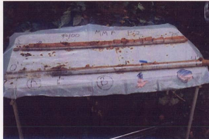
Photo. C-2 Braddock Loam soil profile: surface (A horizon) and subsurface (B horizon) for sample location MMAB2
