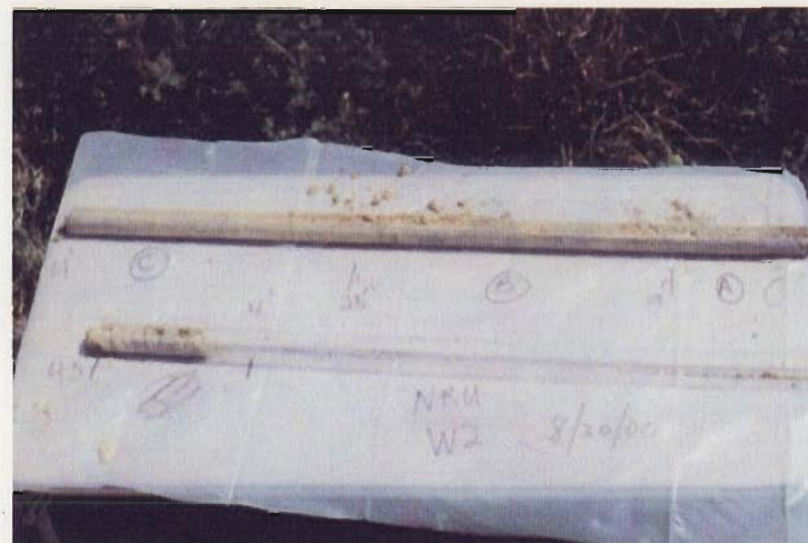
Photo. C-34 Wurno-Newbern-Faywood Silt Loam soil profile: surface (A horizon) and subsurface (B and C horizons) for sample location NRUW2
