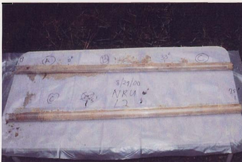
Photo. C-27 Lowell Silt Loam soil profile: surface (A horizon) and subsurface (B and C horizons) for sample location NRUL2
