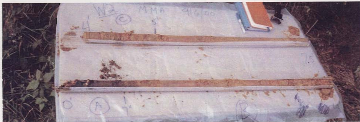
Photo. 6 Wheeling Sandy Loam soil profile for sample location MMAW2: surface (A horizon) and subsurface (B and C horizons) collected from the MMA
