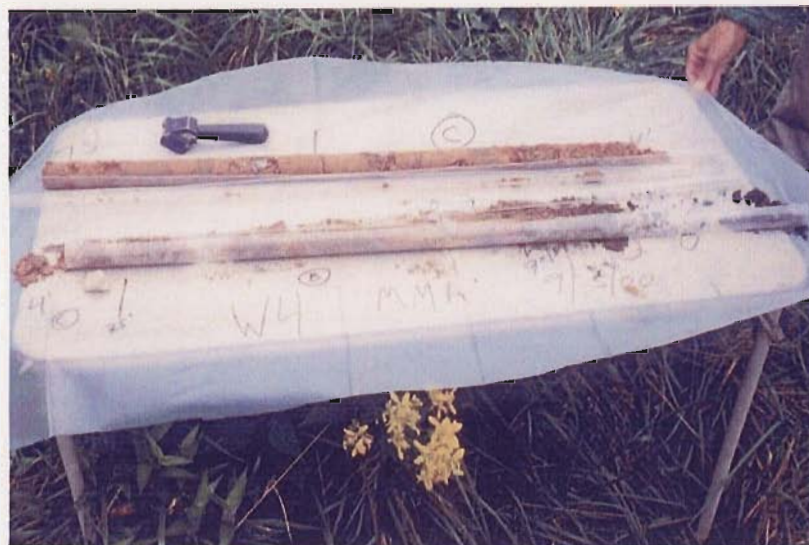
Photo. C-15 Wheeling Sandy Loam soil profile: surface (A horizon) and subsurface (B and C horizons) for sample location MMAW4
