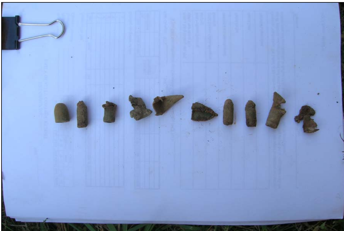
Photograph 3 – Bullets and fragments found within berm approximately 3 to 4 inches bgs
